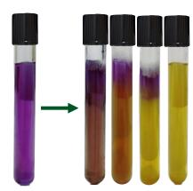
The tubes should be placed in places of the autoclave where it is possible that the sterilization conditions will not be fully established in those areas. For example, the bottom of the autoclave or the middle of it. If it is necessary to autoclave a large volume of materials; For example, flasks containing large amounts of liquid or solid materials, it is necessary to place the bioindicator into the flask or place it next to the equipment.
